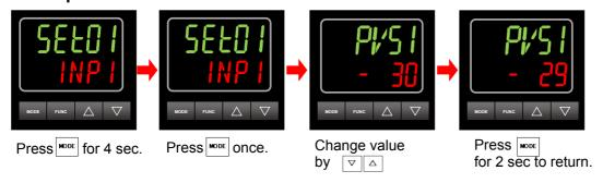
\*If temperature calibration with higher accurancy, leave the soldering unit for 30 minutes,
