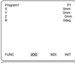
Using JOG key to move iron cartridge until the "pass point of line soldering".
