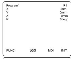
Using JOG key to move iron cartridge until the "pre solder " point.
