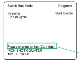
To turn off the buzzer, reset the counter current value while the machine is stopping.
