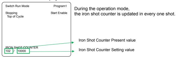
When the present value of the counter reaches the maximum iron shot counter point, the message on teaching pendant appears and a buzzer sounds. (The robot operation enables after reaching set value.)
