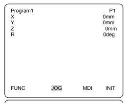
Using JOG key to move iron cartridge until the "Point Soldering (No Up)" point.
