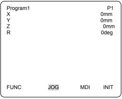
Using JOG key to move iron cartridge until the "end of line soldering" point.
