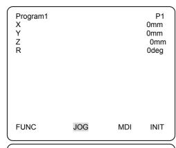
Using JOG key to move iron cartridge until the "cleaning point".
