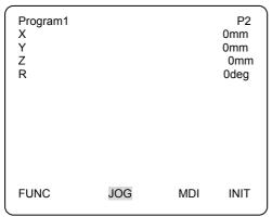
The pass point of line soldering has been registered and the next point screen is displayed.
