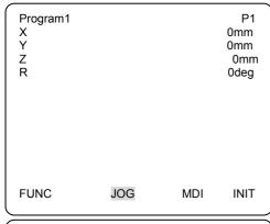
Using JOG key to move iron cartridge until the "PTP Evasion point".
