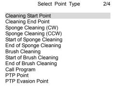
Select the type "Cleaning Start Point" by SEL key. \*Page 2 is displayed by SHIFT+CURSOR key.
