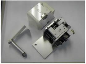
(2) Loosen the set screw "1" for alignment cutting blade shaft and the setting nut "2" to adjust the shaft position. Then move the blade shaft position to match the center of the cutting blade and V grove of the lower roller.
