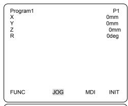
Using JOG key to move iron cartridge until the "arc of line soldering point".
