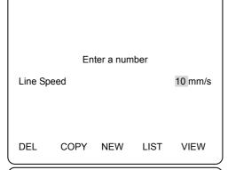
Enter the slide line speed. (Normally 3~10mm/sec setting is recommended.)
