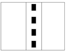
(6) Cut the solder wire with holes perpendicularly and check the cross section. Make sure the cutting blade penetrates into flux core.
