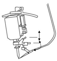
4) Solder wire feeding position can be adjusted.
