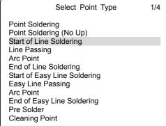
Select the type "Start of Line Soldering" by SEL key.
