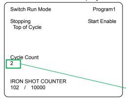
During External operation mode or Switch run mode, it is counted at the time running program ends 1 cycle, then it is displayed on teaching pendant.
