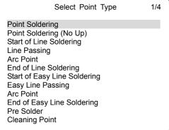
Select the type "Point Soldering" by SEL key.
