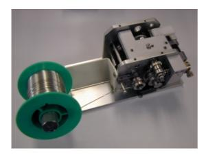
(5) Push down the forward/reverse lever and feed the solder wire, then make sure the cutting blade makes holes on the center of the solder wire. If the holes were not on the center, adjust the cutting blade shaft position, then feed the solder wire and check it.
