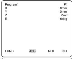
Using JOG key to move iron cartridge until the "Point soldering" point.
