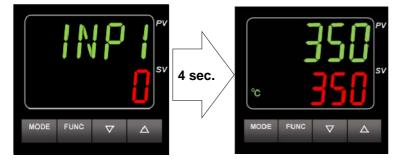
\*When the PV display shows in green color, PV value alarm is within the setting range. When it is in red, it is out of its range.
