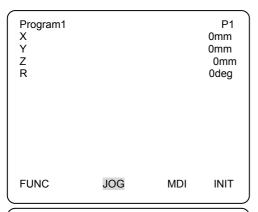
Using JOG key to move iron cartridge until the "start of line soldering" point.
