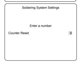
Press CLEAR key to clear the number. It should be done everytime after replacing to new iron cartridge.
