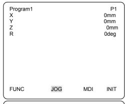
Using JOG key to move iron cartridge until the "cleaning start point".
