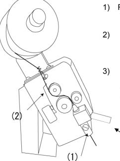
1) Remove the tube and pull solder wire through first. Then attach the solder tube.
